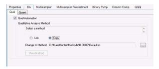
**c** Optional. Click **Quant**. Mark the **Quant Automation** check box. The name of the current Quantitative Analysis method is shown in the list. If you want to change the Quantitative Analysis method that is connected, click \_\_\_\_\_ to select a different method. When the Data Acquisition method is saved, the Quantitative Analysis method that you selected is copied or linked to the Data Acquisition method.
