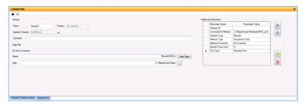
You can run a Data Analysis method from this window by selecting **Both Acquisition and DA** or **DA Only** for the **Method Type**. In addition, you have to set **Override DA method** to indicate which Data Acquisition method contains the DA (Data Analysis) method to execute. You always have to do this.
