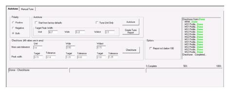
2 Click **Checktune** to evaluate if the MS parameters are within the limits to produce the specified mass accuracy and resolution. Checktune can take approximately 45 minutes.
